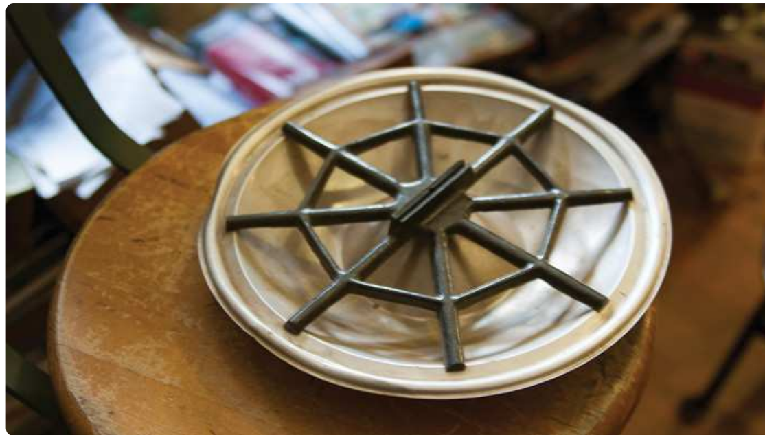
The spider, made with carbon fiber, sends string vibrations from the bridge saddle to numerous points around the resonator cone, both the center and along the edges.
